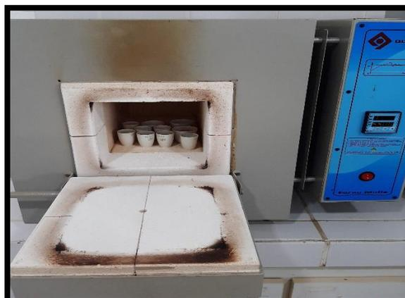
**Figura 10:** Forno Mufla Microprocessado - Q318M QUIMIS<sup>®</sup> com as amostras
