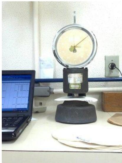
FIGURA 14- Micrômetro REGMED
